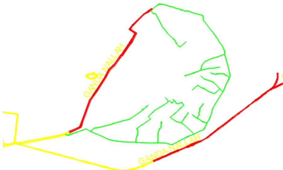
Figure 1-2: Drainage System of Walled City (ABD Area)
